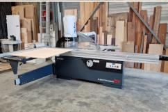
READYtoWORK package of panel saw ITAMAC Maestro X9 3200mm including dust extraction system, extraction hose, clamping bands, mounting clamps etc. and set of main saw blade and scoring blade for finishing sheet panel. Format saws with wide anodised aluminum sliding table on double wear-resistant bar guide with replaceable rollers. Equipped with a built-in module start / stop system which guarantees optimal user comfort.
