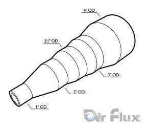
Reducer fitting to be used with the different models of Air Flux Dust extractors. Can be cut off on the appropriate diameter.
