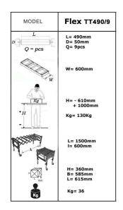
The TT490-9 is a foldable roller bed with 9 rollers on wheels that can be folded in and out in no time. As a result, it can be moved and stored quickly and easily, and will save considerable space in your workshop.
