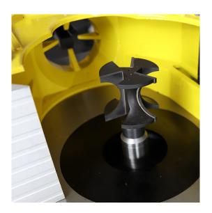
This adaptor is specifically designed to allow router bits to be used on your spindle moulder TT3085/4. Because this adaptor sinks under the work table, your router bit is at the same height as the table. Thus, no further attachments are required for passing the cutter with your workpiece. Combine with the right collet for your router bit. Collets available with Ø8, 10 or 12mm.
