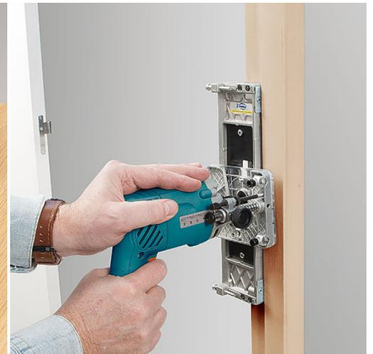
Specially designed for cutting holes for door hinges without using an additional template. It is equipped with a millimetric knob that allows easy adjustment. It can also be used for trimming edges and making slots in wood or plastic. It is also possible to cut mortises with templates, using special base with copier, included in standard equipment. Suitable for working with composite panels (Alucobond® and similar) using routing and folding method (optional 90° and 135° bits).
