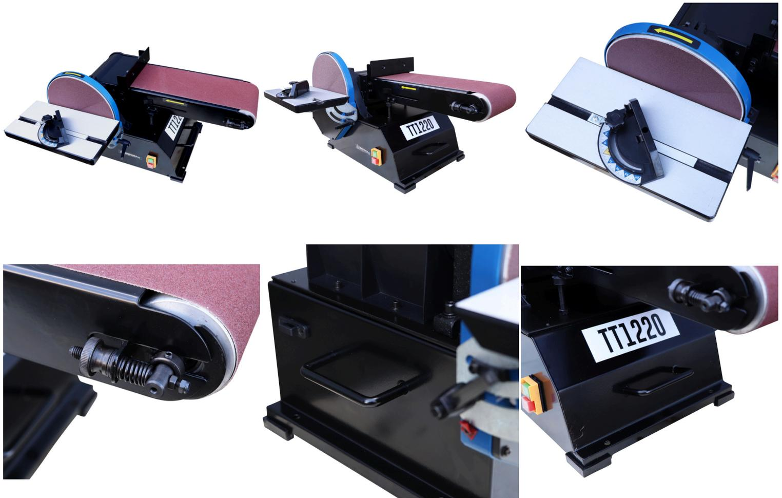
The sander TT1220 can be used vertically, horizontally or at any angle. The large aluminium table can be tilted up to 45° and is equipped with a protractor. The work table is supported on both sides for precision use. It features a D handle for easy transport, and a quick-release sanding belt system for quick changes. The belt can be easily balanced thanks to the handy control knob. The machine also has a 60 mm extraction outlet.
