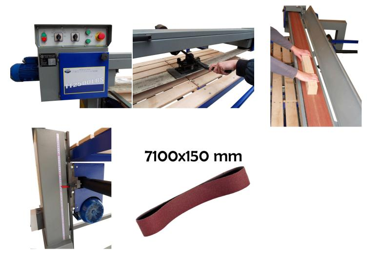
This sander comes standard with 2 sanding speeds. It is both left and right-turning and equipped with an electric (automatic) height adjustment of the sanding table. The machine has 3 motors: for the belt (2 speeds), the height adjustment of the table and the extraction unit. The sturdy and heavy duty construction of the frame ensures good stability. The table can be moved over the steel guides.
