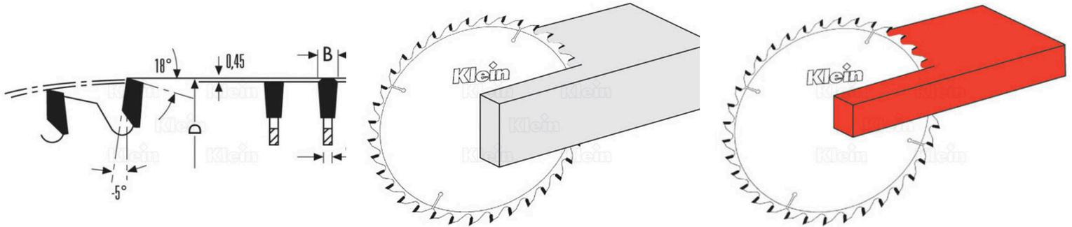
Saw blade 'Xtra Cut' with FZ/TR triple chip teeth and a negative hook angle of 5°. This saw blade is well suited for the cutting of solid aluminium, PVC and non-ferro metals. To be used on table saws. These saw blades offer great finish and longer life. No-noise and less vibration thanks to a special synthetic resin filled in the slots to increase the stability and reduce vibrations. No noise.
