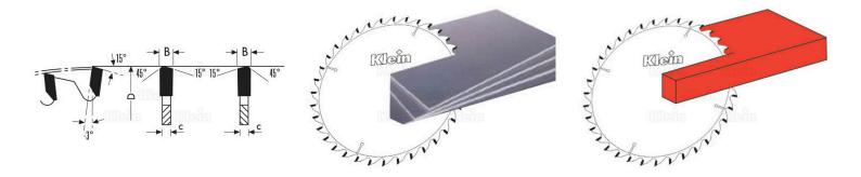
Saw blade with innovative alternate trap teeth (WZ/FA) and a 3° negative hook angle. This saw blade is well suited for cutting of thin plastics, acrylics (plexiglass), PVC or plywood. No noise.
