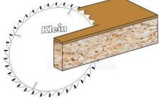
Universal saw blade with alternate top bevel teeth, suited for cutting of different wood types or wooden panels. Make sure to use the right amount of teeth to achieve optimal results of your project. A low number of teeth is suited for fast-paced and rough sawing of solid wood. A high number of teeth calls for a lower operating speed but guarantees a clean cut of both solid wood and wood panels.
