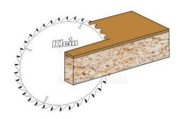
Universal saw blade with alternate top bevel teeth, suited for cutting of different wood types or wooden panels. Make sure to use the right amount of teeth to achieve optimal results of your project. A low number of teeth is suited for fast-paced and rough sawing of solid wood. A high number of teeth calls for a lower operating speed but guarantees a clean cut of both solid wood and wood panels.
