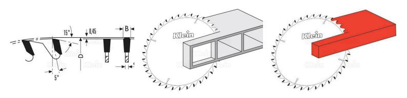
Saw blade 'Xtra Cut' with FZ/TR 'triple chip' teeth and a positive hook angle of 5°. This saw blade is suited for use with aluminium (hollow), PVC and non-ferro metals and can be used for cutting of aluminium profiles and extrusions with a thickness between 2 and 5mm. To be used on table saws. These saw blades offer great finish and longer life. No-noise and less vibration thanks to a special synthetic resin filled in the slots to increase the stability and reduce vibrations. No noise.
