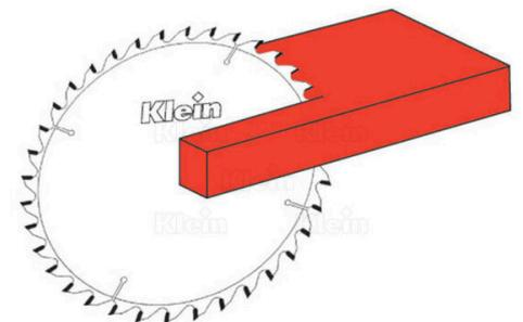
Saw blade 'Xtra Cut' with FZ/TR 'triple chip' teeth and a positive hook angle of 5°. This saw blade is suited for use with aluminium (hollow), PVC and non-ferro metals and can be used for cutting of aluminium profiles and extrusions with a thickness between 2 and 5mm. To be used on table saws. These saw blades offer great finish and longer life. No-noise and less vibration thanks to a special synthetic resin filled in the slots to increase the stability and reduce vibrations. No noise.
