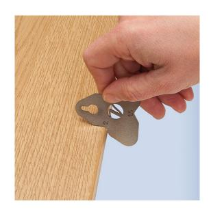
To remove glue residues or burrs and achieve a professional finish. It can cut straight edges or edges with a radius of 1 - 1.5 - 2 mm. Highly resistant and durably treated steel. Special surface coating to prevent corrosion.
