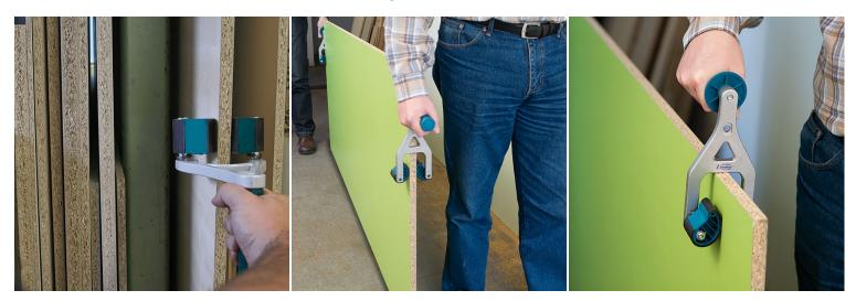
With its ergonomic shape, this handle helps you to easily transport panels in different materials. The handle has three basic functions: pulling, carrying or lifting. Thanks to its aluminium design, this handle is very strong and robust. The maximum load is 70kg. Suitable for panels between 0mm and 46mm thick.
