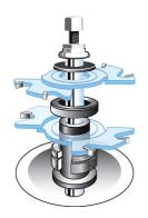
A set of six spacers of high quality with a tolerance of 0.01. Machined using the fineblanking process. All spacers are bore diameter 50mm and outer diameter 70mm The thickness varies between 2mm and 30mm.
