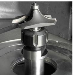
This set offers you a ready-to-use solution to mount router bits with shank Ø8mm, Ø10mm or Ø12mm on your spindle moulder machine. Thanks to the M14 shaft, the concentric chuck can be quickly and easily fitted to the spindle of your milling machine. Combine with one of the three spring collets to obtain the correct diameter to fit your router bit.
