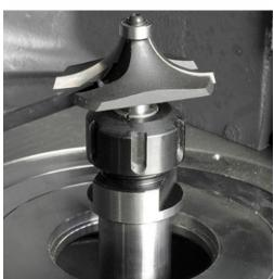
This set offers you a ready-to-use solution to mount router bits with shank Ø6mm, Ø8mm or Ø12mm on your spindle moulder machine. Thanks to the M16 shaft, the concentric chuck can be quickly and easily fitted to the spindle of your milling machine. Combine with one of the three spring collets to obtain the correct diameter to fit your router bit.
