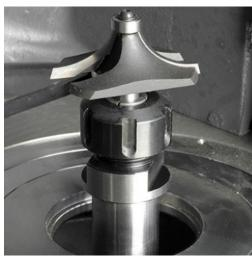
This set offers you a ready-to-use solution to mount router bits with shank Ø8mm, Ø10mm or Ø12mm on your spindle moulder machine. Thanks to the M16 shaft, the concentric chuck can be quickly and easily fitted to the spindle of your milling machine. Combine with one of the three spring collets to obtain the correct diameter to fit your router bit.
