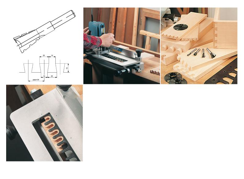
Convenient all in one set to make dovetail joints with the Virutex PL11. The set includes an interchangeable PVC mould with tooth spacing (pas) 34mm, an adapted guide ring Ø23mm and the correct dovetail bit Ø19mm. Use this set to make large dovetail joints (e.g. for furniture). Minimum thickness of the wood to be able to work correctly is 24mm.
