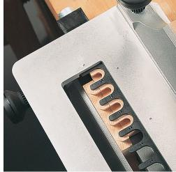
Convenient all in one set to make dovetail joints with the Virutex PL11. The set includes an interchangeable PVC mould with tooth spacing (pas) 34mm, an adapted guide ring Ø23mm and the correct dovetail bit Ø19mm. Use this set to make large dovetail joints (e.g. for furniture). Minimum thickness of the wood to be able to work correctly is 24mm.
