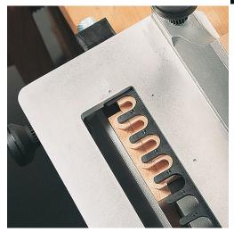
Convenient all in one set to make dovetail joints with the Virutex PL11. The set includes an interchangeable PVC mould with tooth spacing (pas) 16mm, an adapted guide ring Ø12mm and the correct dovetail bit Ø9,5mm. Use this set to make small dovetail joints (e.g. for jewellery boxes). Minimum thickness of the wood to be able to work correctly is 11mm.
