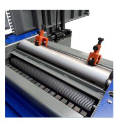
This handy tool allows you to adjust your planing knives or planing bits quickly, easily and precisely. With the help of the magnets, the tool fixes itself on the shaft. You can then place the planing knive in the correct position in no time at all. Standard delivery in a neat wooden case.
