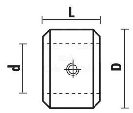
Rings for setting the drilling depth use when working with manual feed. Used with Art. R101 - R201 - R205.
