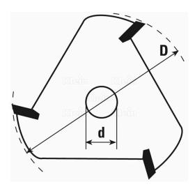
These slot cutters are suitable for a wide range of applications. Quickly and easily cut the right pen and groove connections for your project. The different cutting lengths of the cutters ensure that you always get the correct thickness of your pins or slots. Thanks to its cutting edges in high-quality carbide (widia), this cutter cuts through most types of wood without any problems.
