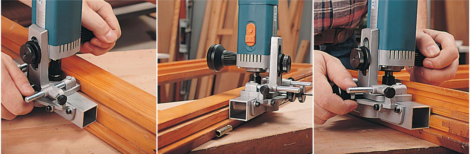
Specially designed for slotting doors and windows. Thanks to this milling cutter it is possible to insulate without disassembling your joints. Place rubbers or other seals to insulate your window or doors efficiently. Perfect for installing Virutex rubber or PVC seals.
