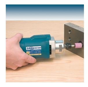
Straight grinder, equipped as standard with 6mm collet, for metal finishes and rough machining. Collets of other sizes are available on request. Easily combine this grinder with most standard grinding accessories on the market. Equipped with electronic speed control. Thanks to the standard collar of 43mm, you can also use this machine as a motor for milling work, for example.
