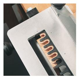
This straight cutter is suitable for making straight grooves for box joints. Use these joints to construct cabinet drawers, coffins, cases, or other types of furniture. Thanks to the hard metal (carbide) cutting edges, a clean and accurate result of all your milling and woodworking projects is guaranteed.
