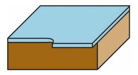
Klein® trimming bits with straight cut are suitable for smooth and well-finished edges on melamine and veneered panels. The ball bearing, having the same diameter of the cutters, trims any overlap leaving a flat and smooth edge. Two flutes provide fast cutting and good chipping ejection.
