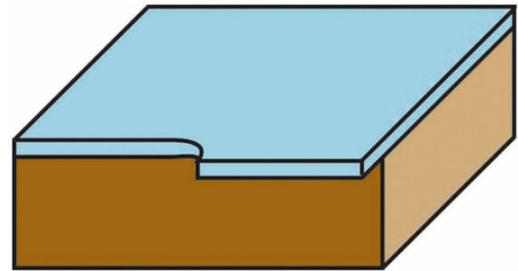
Klein® trimming bits with straight cut are suitable for smooth and well-finished edges on melamine and veneered panels. The ball bearing, having the same diameter of the cutters, trims any overlap leaving a flat and smooth edge. Two flutes provide fast cutting and good chipping ejection.
