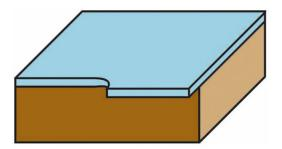
Klein® trimming bits with straight cut are suitable for smooth and well-finished edges on melamine and veneered panels. The ball bearing, having the same diameter of the cutters, trims any overlap leaving a flat and smooth edge. Two flutes provide fast cutting and good chipping ejection. The blades are specially sheared so you can work faster and splinter free.
