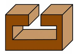
This router bit is specially made for creating T-slots in most types of wood. These can be used, among other things, to fit aluminium profiles. The router bit in high-quality carbide (widia) guarantees you a perfect finish for all your projects.
