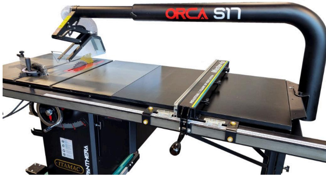
The saw table insert is designed for use at any cutting angle and can be easily removed thanks to the **magnetic attachment** in the table. Through fine adjustment, this plate can also be adjusted for a 100% flat transition with the cast-iron table top.
