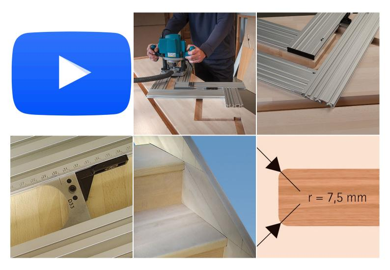
Template for open and closed staircases. Easy and fast to use with three functions in one. Milling both the groove for the step, counter step, and stair nose thanks to this template. The template is reversible and can be used for both the left and right side of the stairs. Supplied as standard with one stair nose Radius 7.5, other stair noses available on request. The stair thickness is adjustable between 18-55mm using the supplied templates.
