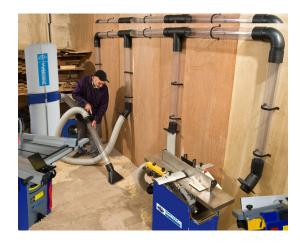
Tubes are more efficient than hoses for long distance dust collection. This clear plastic tube is available in 100cm lengths to get your dust from point A to point B. Use 100mm extraction hose or connector (art. 3DU1070) to join pipes together, or to connect the pipe to other 100mm accessories.
