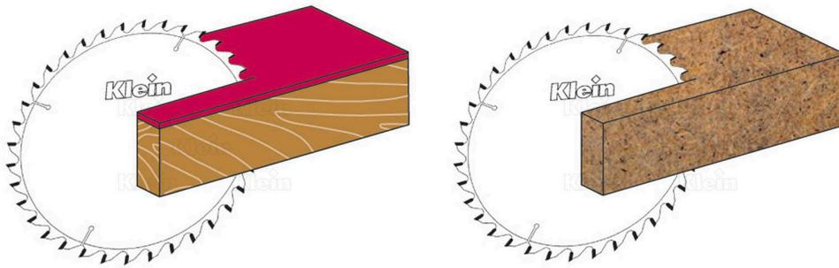
Trimming and sizing saw blade 'Xtra Cut' with FZ/TR triple chip trapezoidal teeth, suited for the cutting of hardwoods, double sided veneer and laminate board, MDF, hard paper and thermoplastic boards. To be used on table saws. These saw blades offer great finish and longer life. No-noise and less vibration thanks to a special synthetic resin filled in the slots to increase the stability and reduce vibrations.
