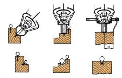
Two-sided straight bit to be used on the Virutex RA17VG slotting machine. This bit makes it possible to mill in silicone seals type FS1 or FS3.
