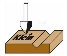
These V-grooving router bits allow you to make deep and shallow V-groove, ideal for sign-making or for decorative features on panels or furniture. Use these router bits with no risk of burning. They are suitable also for making 90° chamfer. It is recommended to pass multiple times when removing large quantities of material.
