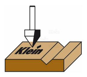
These V-grooving router bits allow you to make deep and shallow V-groove, ideal for sign-making or for decorative features on panels or furniture. Use these router bits with no risk of burning. They are suitable also for making 90° chamfer. It is recommended to pass multiple times when removing large quantities of material.
