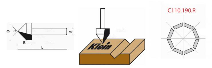
These V-grooving router bits allow you to make deep and shallow V-groove, ideal for sign-making or for decorative features on panels or furniture. Use these router bits with no risk of burning. They are suitable also for making 90° chamfer. It is recommended to pass multiple times when removing large quantities of material.
