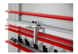
The Verticut TT1632 WPM is a space-saving vertical panel saw for 3200 by 1600 mm panels.
