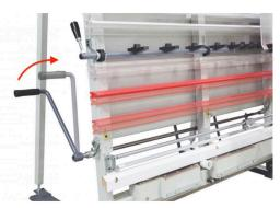
The Verticut TT1225 WPM is a space-saving vertical panel saw for panels of 2500 x 1220 mm.
