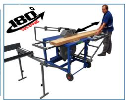
This Timber Yard Champ TT400TX with a 180° rotating table is the perfect saw table for construction and contracting companies. This is the ideal machine for the construction of, for example, carports, garden sheds and dog houses, canopies, etc.
